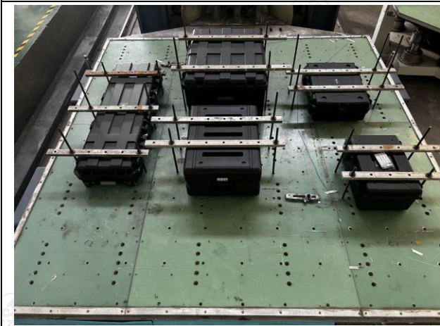
Fig.2-5 Test erection (X-axis)
