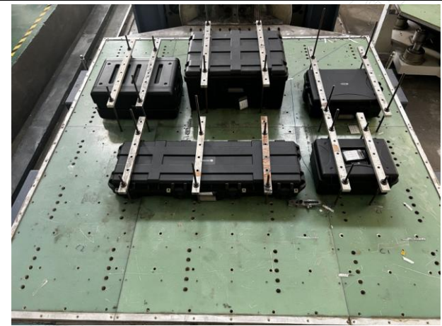
Fig.2-4 Test erection (Y-axis)
