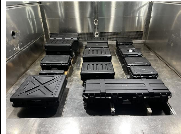
Fig.1-3 Low temperature test erection
