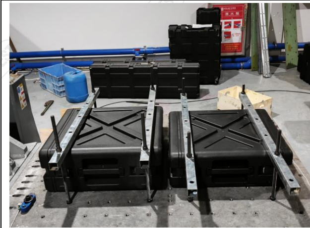
Fig.2-3 Vibration Test Subject Installation Status - X-Axis
