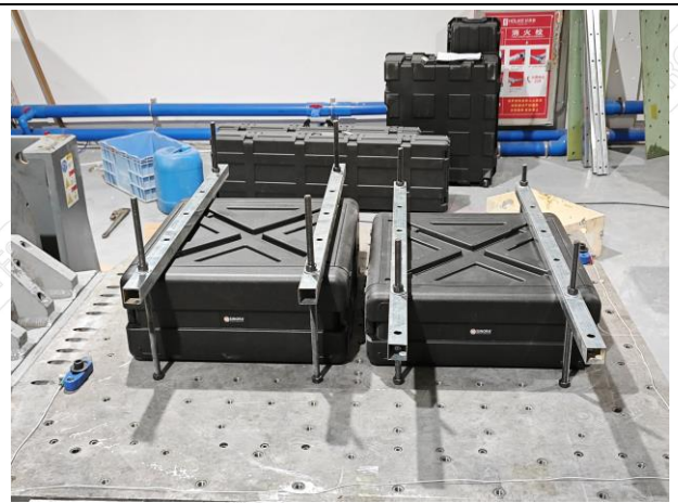
Fig.2-6 Vibration Test Subject Installation Status - Y-Axis
