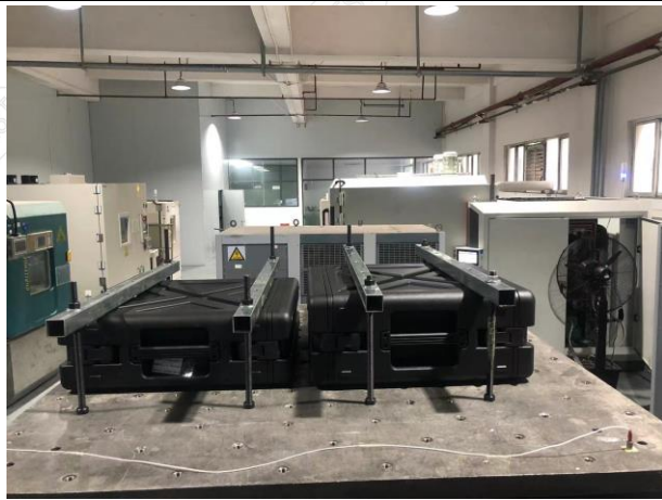
Fig.2-9 Vibration Test Subject Installation Status - Z-Axis
