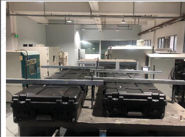
Fig.2-9 Vibration Test Subject Installation Status - Z-Axis
