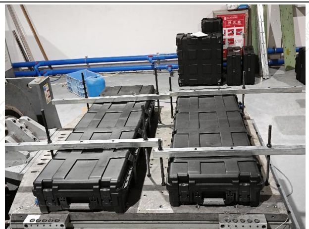
Fig.2-6 Vibration Test Subject Installation Status - Y-Axis
