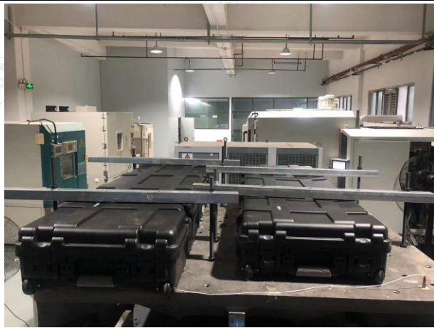
Fig.2-9 Vibration Test Subject Installation Status - Z-Axis
