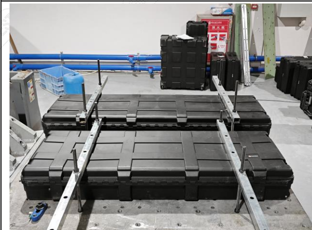
Fig.2-3 Vibration Test Subject Installation Status - X-Axis
