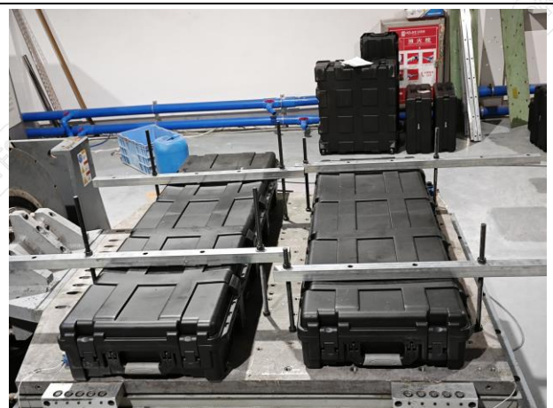
Fig.2-6 Vibration Test Subject Installation Status - Y-Axis
