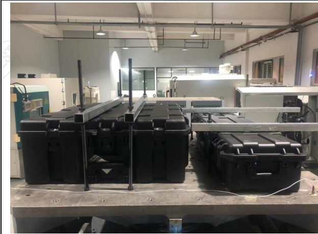
Fig.2-9 Vibration Test Subject Installation Status - Z-Axis
