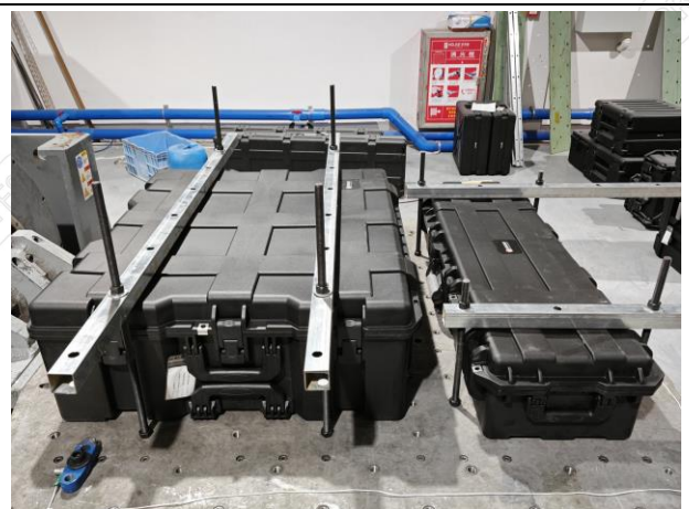
Fig.2-6 Vibration Test Subject Installation Status - Y-Axis
