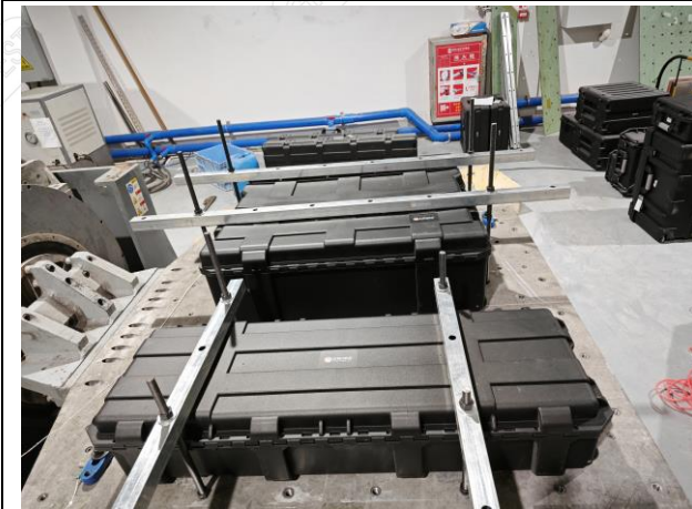
Fig.2-3 Vibration Test Subject Installation Status - X-Axis
