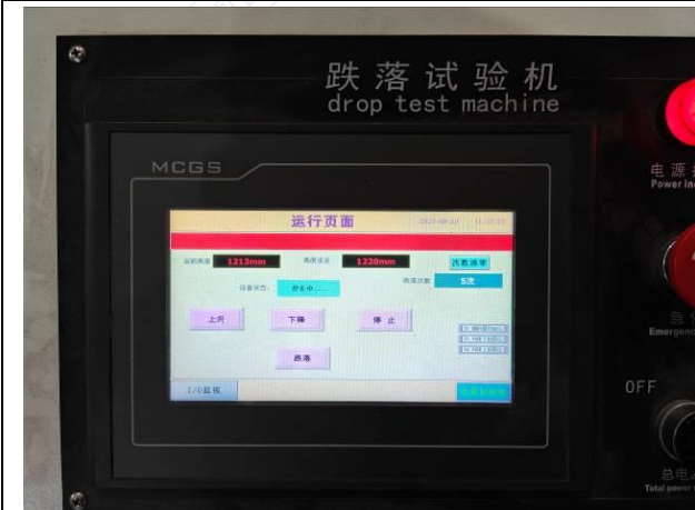
Fig.3-3 Operation Diagram Of Drop Testing Machine Interface
