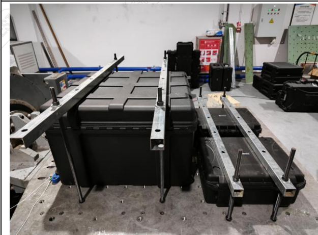
Fig.2-3 Vibration Test Subject Installation Status - X-Axis
