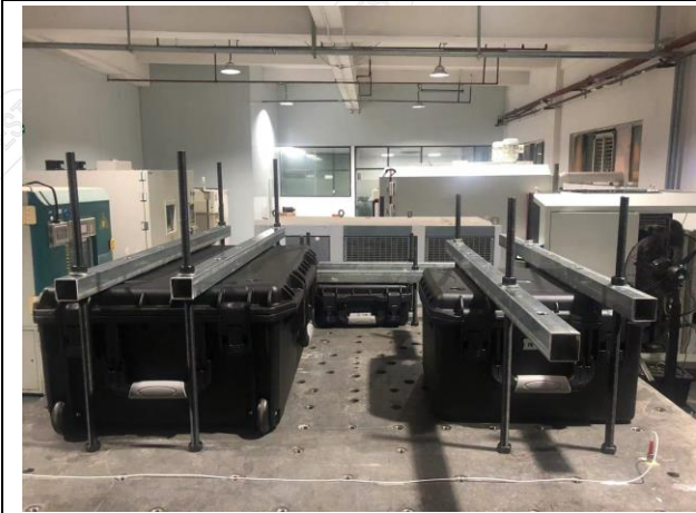
Fig.2-9 Vibration Test Subject Installation Status - Z-Axis
