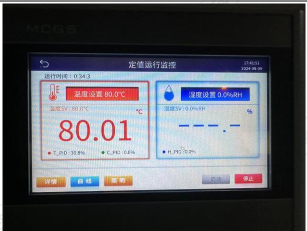
Fig.1-6 High Temperature Test Operation Interface Diagram
