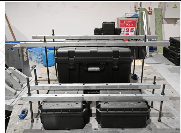
Fig.2-6 Vibration Test Subject Installation Status - Y-Axis
