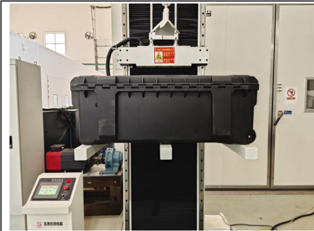
Fig.3-5 Drop test Operation - Surface Schematic Diagram
