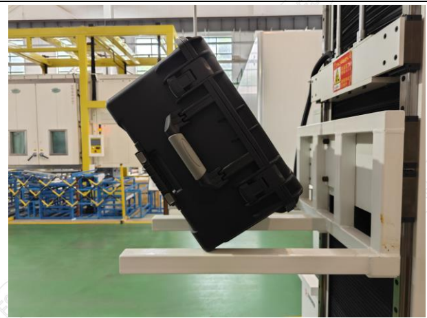
Fig.3-6 Drop Test Operation - Edge Diagram
