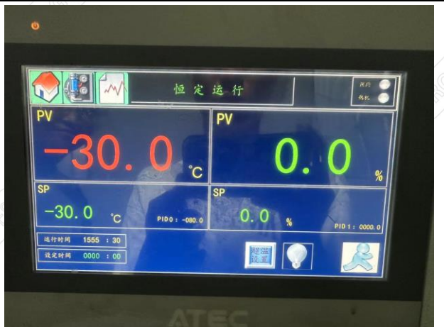
Fig.1-4 Low Temperature Test Operation Interface Diagram
