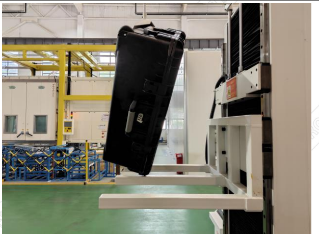
Fig.3-4 Drop Test Operation - Angle Diagram
