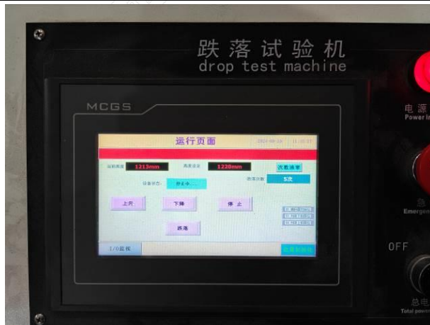
Fig.3-4 Operation Diagram Of Drop Testing Machine Interface
