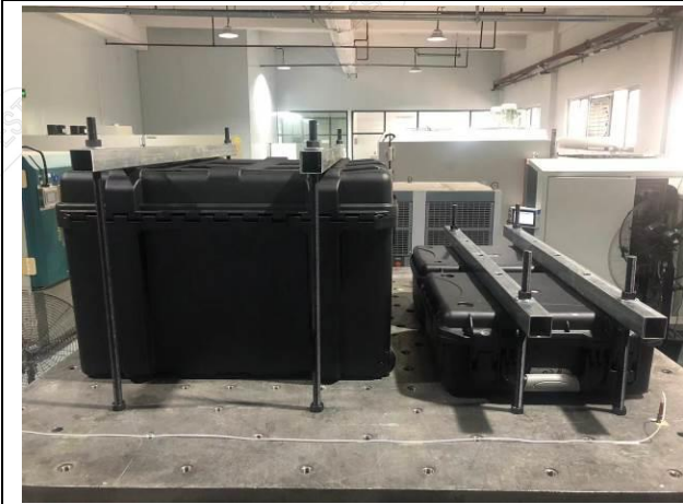
Fig.2-9 Vibration Test Subject Installation Status - Z-Axis
