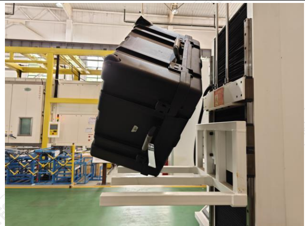
Fig.3-5 Drop Test Operation - Angle Diagram
