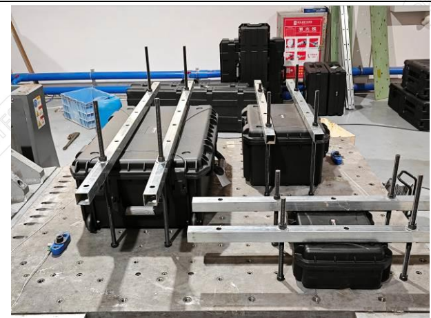
Fig.2-6 Vibration Test Subject Installation Status - Y-Axis
