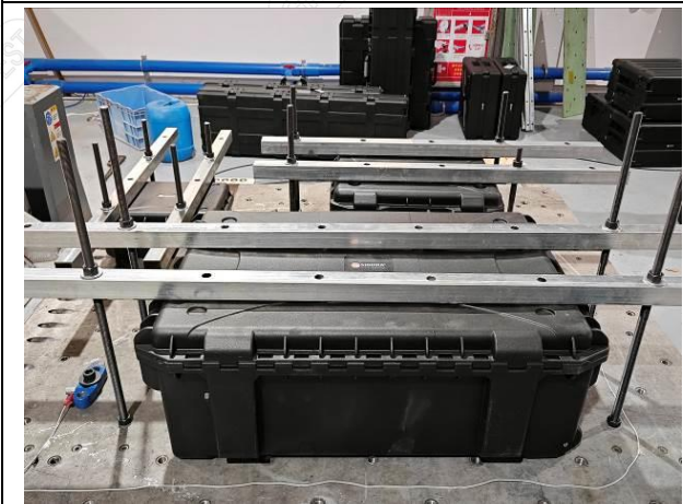
Fig.2-3 Vibration Test Subject Installation Status - X-Axis
