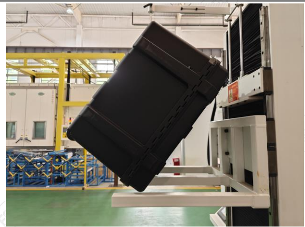
Fig.3-7 Drop Test Operation - Edge Diagram
