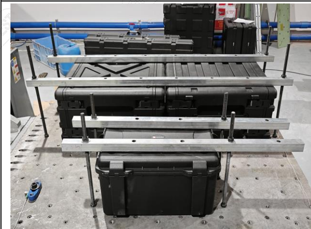
Fig.2-3 Vibration Test Subject Installation Status - X-Axis
