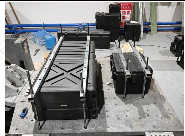
Fig.2-6 Vibration Test Subject Installation Status - Y-Axis
