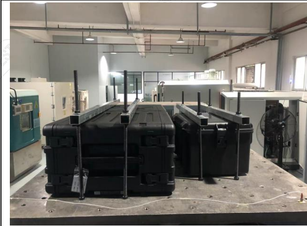
Fig.2-9 Vibration Test Subject Installation Status - Z-Axis
