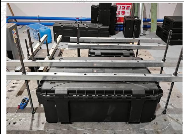
Fig.2-3 Vibration Test Subject Installation Status - X-Axis
