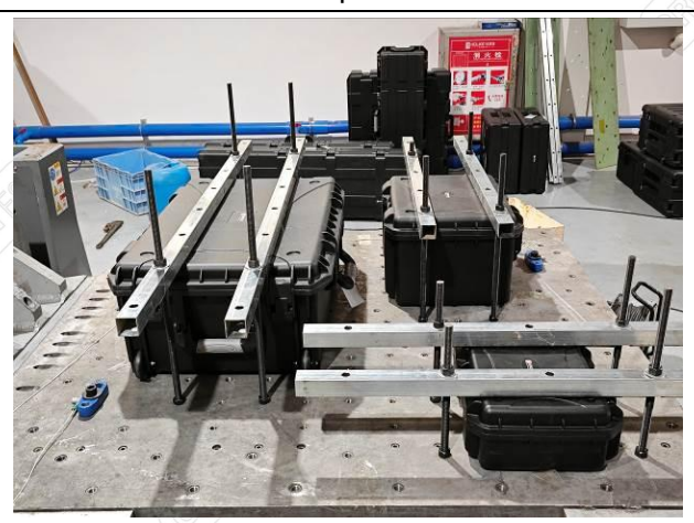
Fig.2-6 Vibration Test Subject Installation Status - Y-Axis
