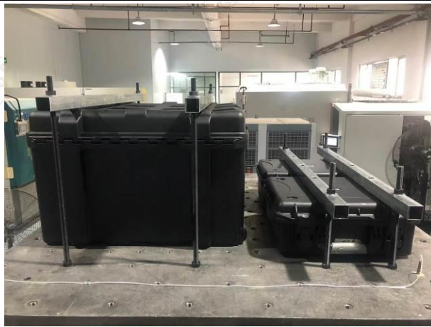
Fig.2-9 Vibration Test Subject Installation Status - Z-Axis
