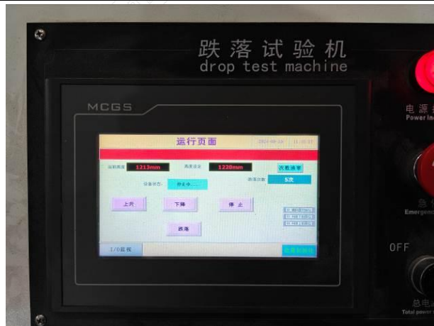
Fig.3-3 Operation Diagram Of Drop Testing Machine Interface
