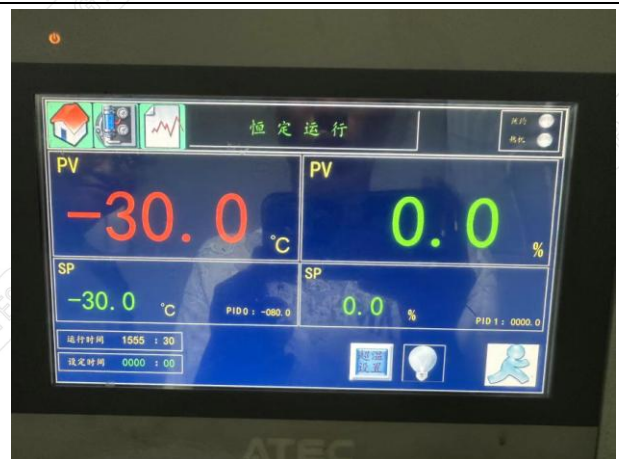
Fig.1-4 Low Temperature Test Operation Interface Diagram
