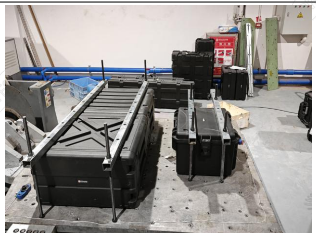
Fig.2-6 Vibration Test Subject Installation Status - Y-Axis
