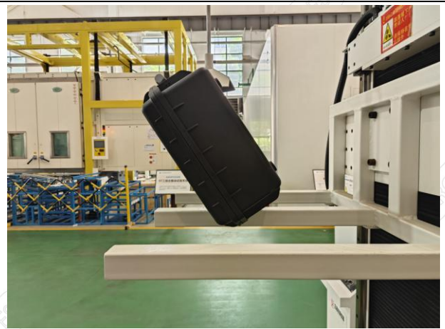
Fig.3-6 Drop Test Operation - Edge Diagram
