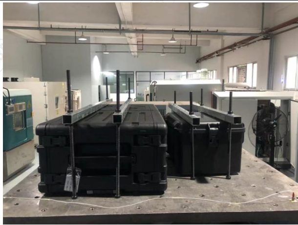
Fig.2-9 Vibration Test Subject Installation Status - Z-Axis
