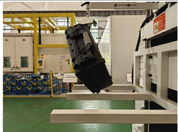
Fig.3-4 Drop Test Operation - Angle Diagram
