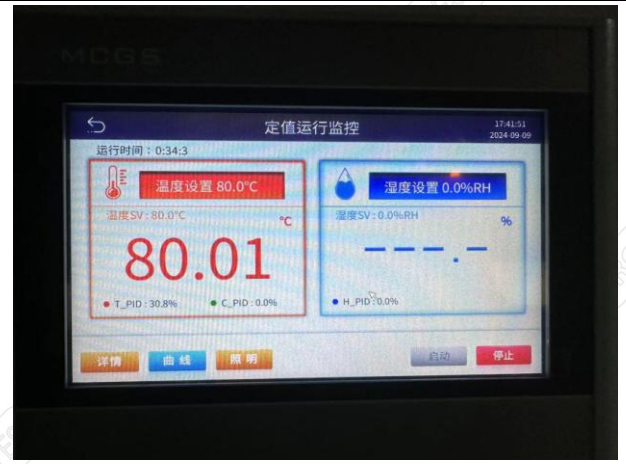
Fig.1-6 High Temperature Test Operation Interface Diagram
