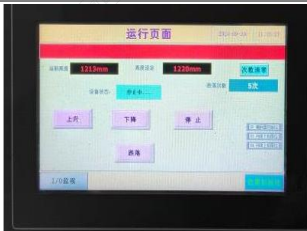
Fig.3-3 Operation Diagram Of Drop Testing Machine Interface
