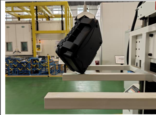
Fig.3-5 Drop test Operation - Surface Schematic Diagram
