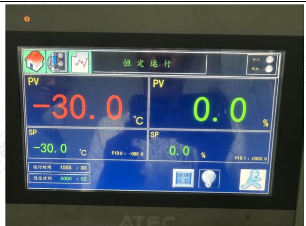
Fig.1-4 Low Temperature Test Operation Interface Diagram
