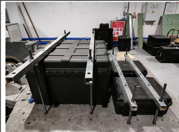
Fig.2-3 Vibration Test Subject Installation Status - X-Axis
