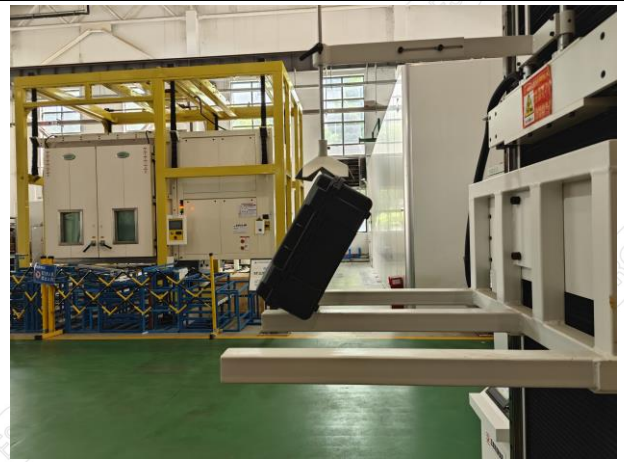
Fig.3-6 Drop Test Operation - Edge Diagram
