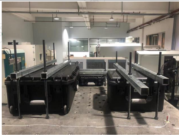
Fig.2-9 Vibration Test Subject Installation Status - Z-Axis
