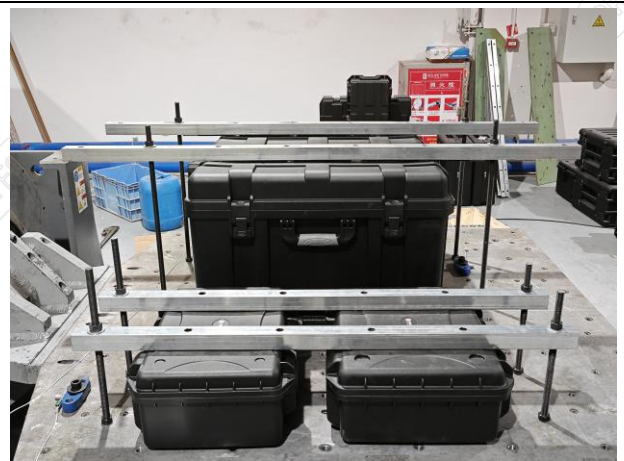
Fig.2-6 Vibration Test Subject Installation Status - Y-Axis
