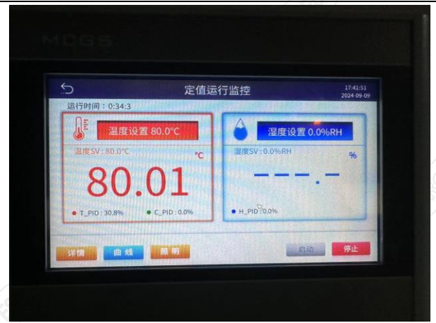
Fig.1-6 High Temperature Test Operation Interface Diagram
