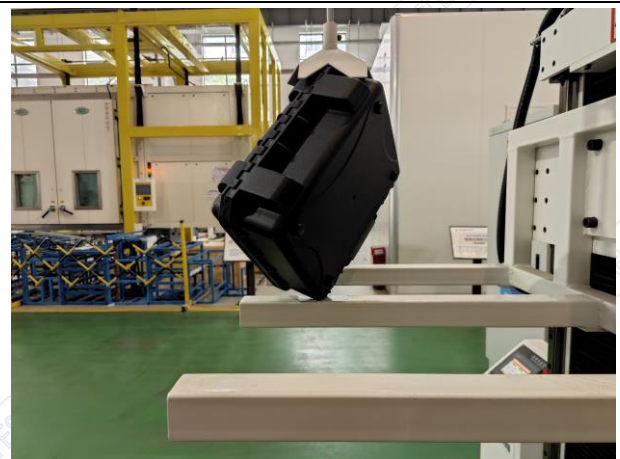
Fig.3-4 Drop Test Operation - Angle Diagram
