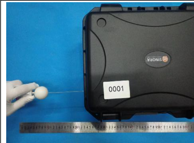
Fig.1-3 Pre-test metal probe inspection
