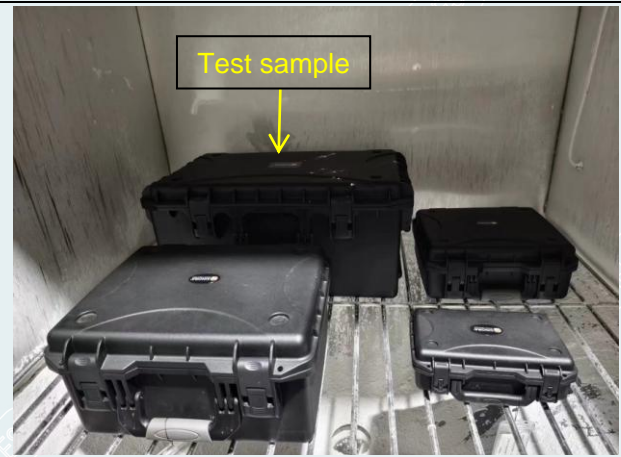
Fig.1-6 Test sample placement
