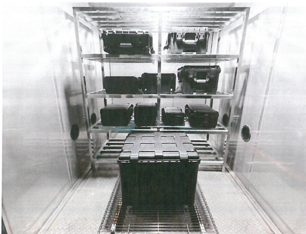
Attached figure 2.3 Temperature impact test subject placement diagram (H202312204372-0010)
