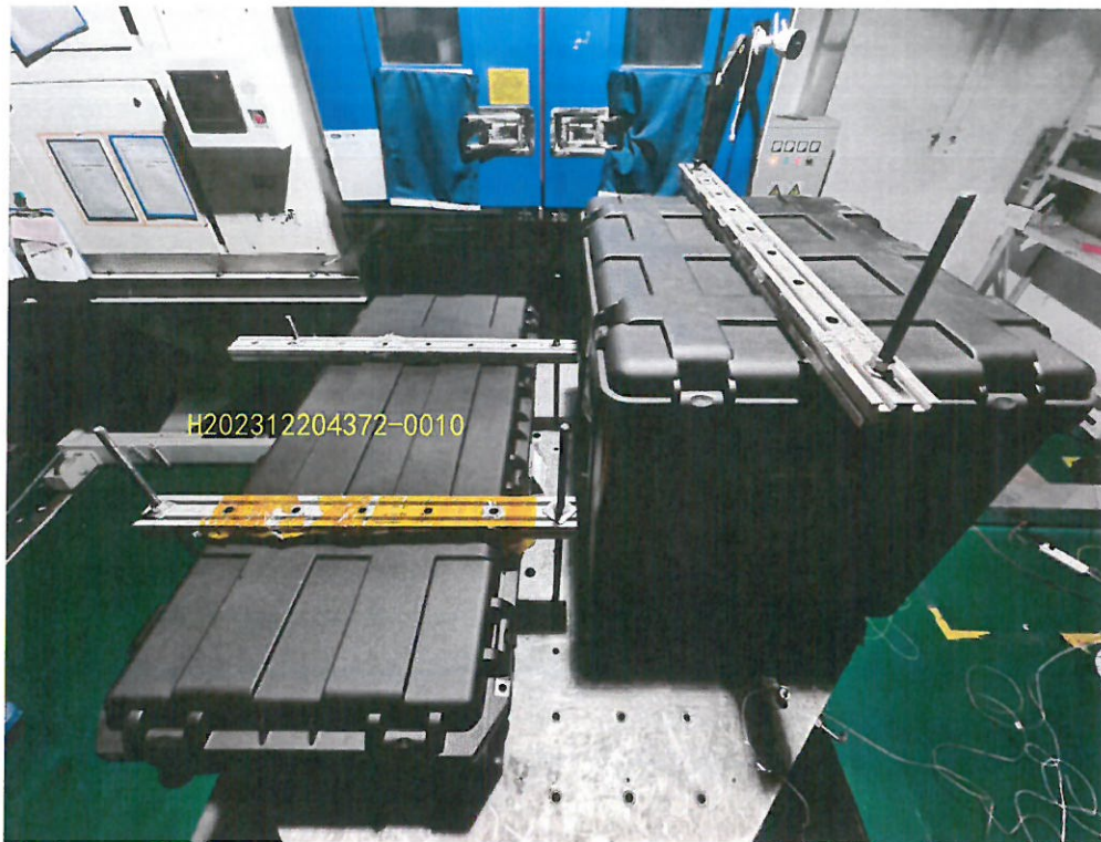
Attached figure 2.7 The vibration test is typically set up by the sample-Z axis (H202312204372-0010)
