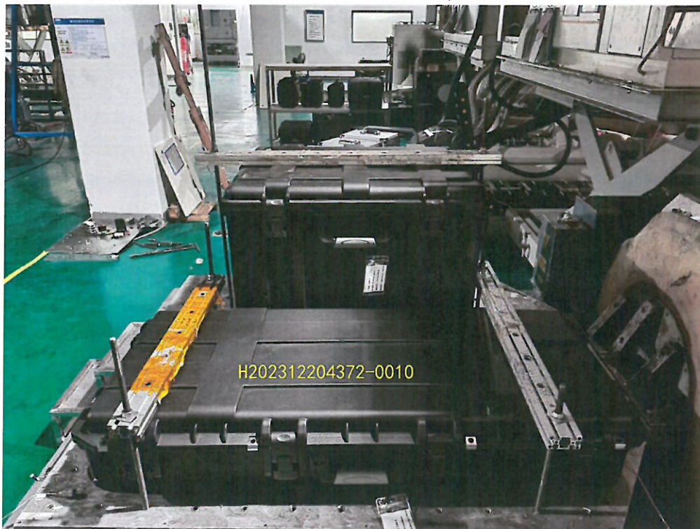
Attached figure 2.6 The vibration test is typically set up by the sample-X axis (H202312204372-0010)
