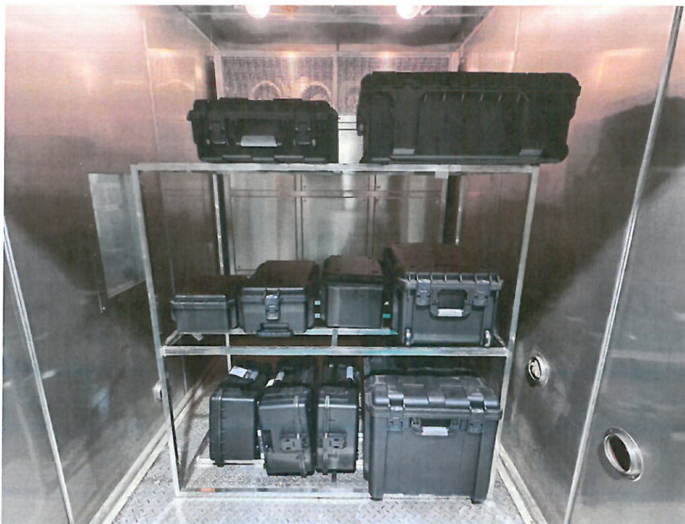
Attached figure 2.1 Temperature shock test subject placement diagram (H202312204372-00100)
