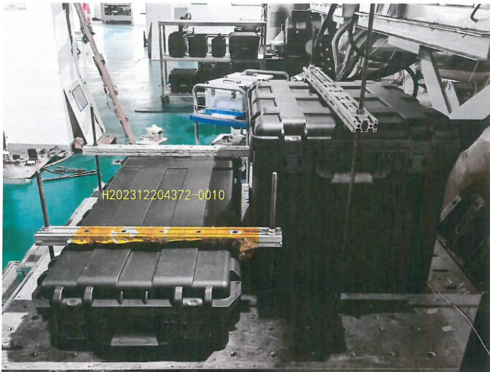
Attached figure 2.5 The vibration test is typically set up by the sample-Y axis (H202312204372-0010)
