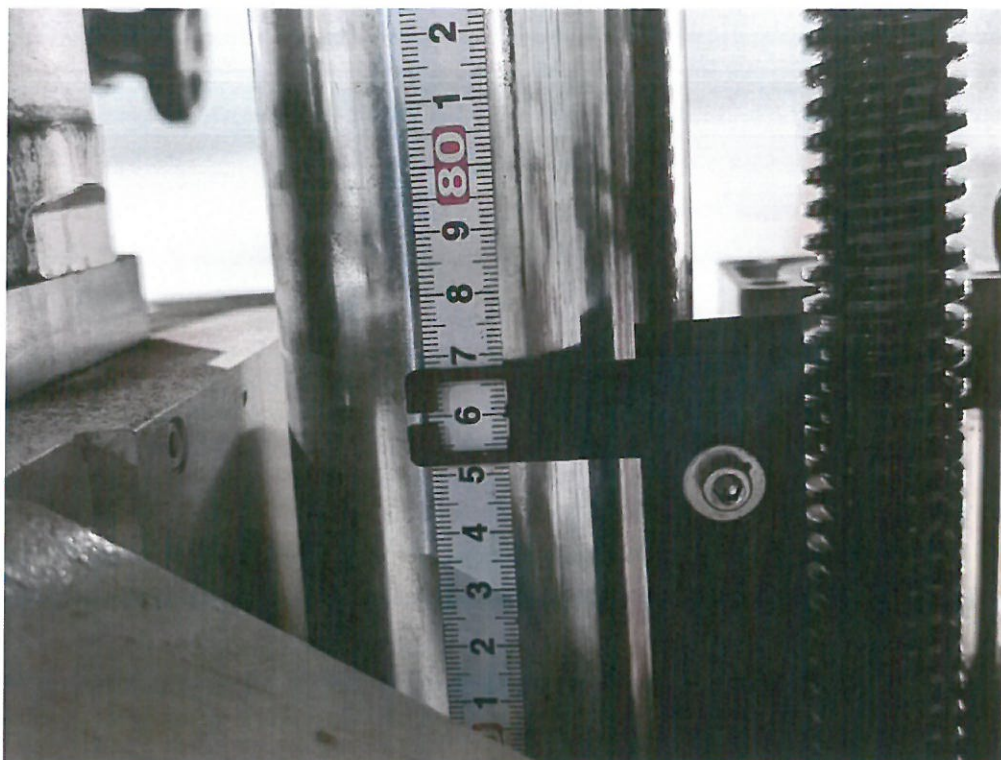
Attached figure 2.17 drawing of drop height 76cm (H202312204372-0010)
