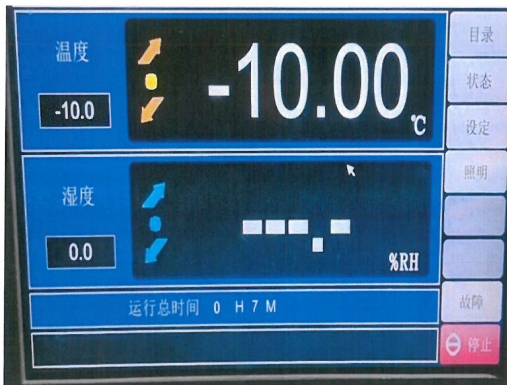
Attached figure 2.4 Temperature shock test equipment running interface-cryogenic box (H202312204372-0010)
