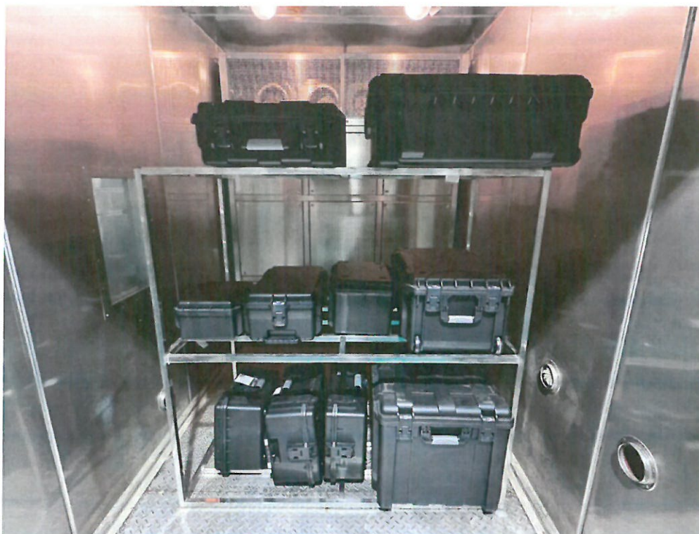
Attached figure 2.1 Temperature shock test subject placement diagram (H202312204372-0009)
