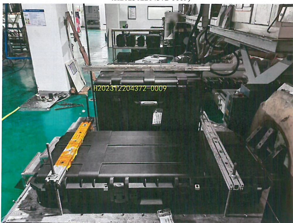
Attached figure 2.6 The vibration test is typically set up by the sample-X axis (H202312204372-0009)
