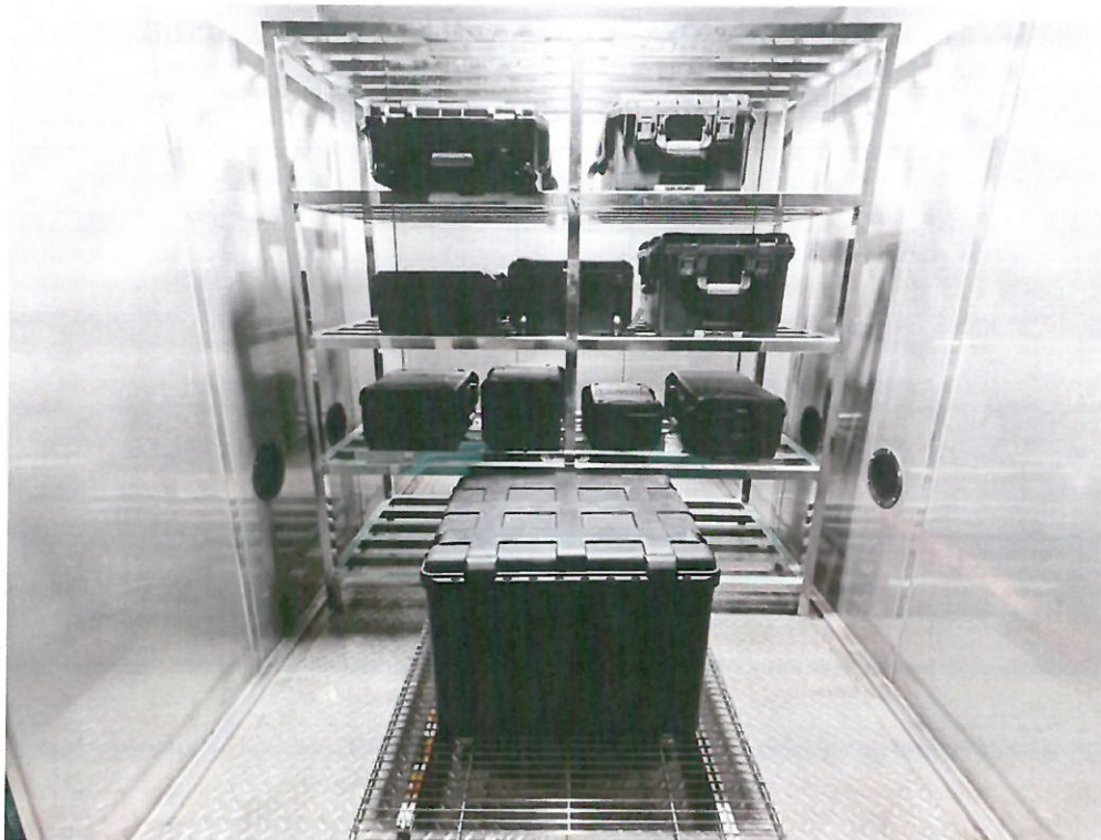
Attached figure 2.3 Temperature impact test subject placement diagram (H202312204372-0009)
