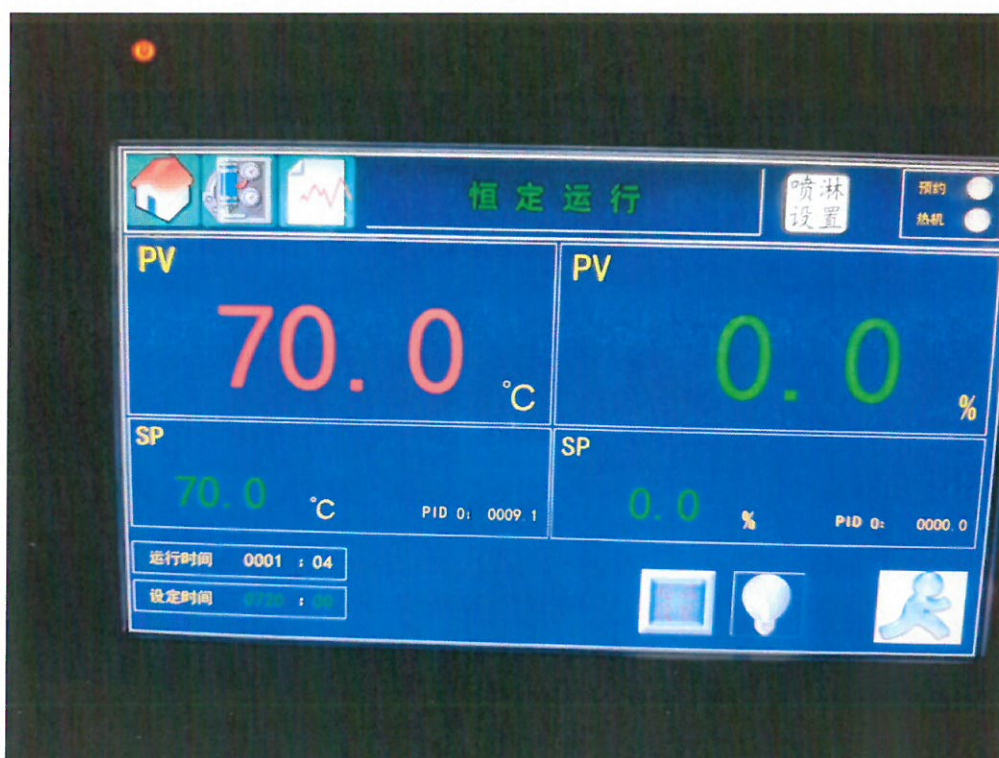
Attached figure 2.2 Temperature shock test equipment running interface - high temperature box (H202312204372-0009)
