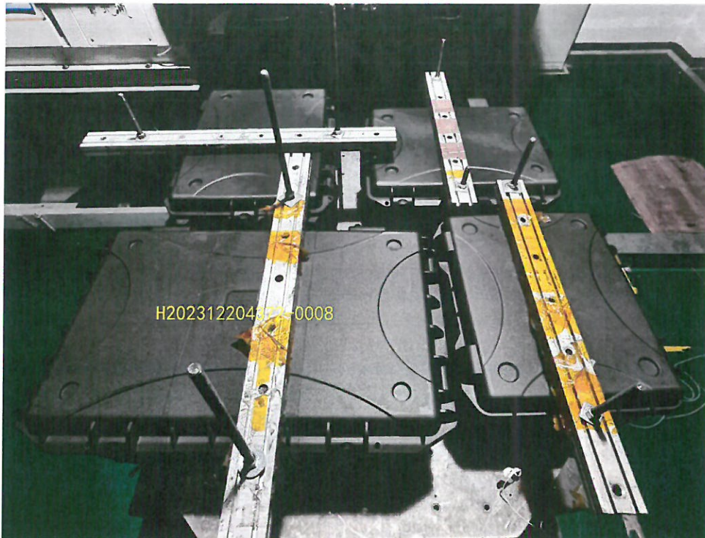
Attached figure 2.7 The vibration test is typically set up by the sample-Z axis (H202312204372-0008)
