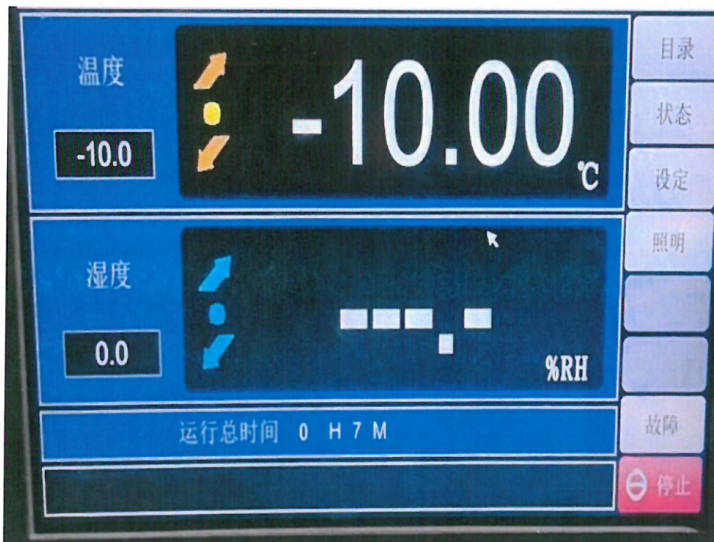
Attached figure 2.4 Temperature shock test equipment running interface-cryogenic box (H202312204372-0008)
