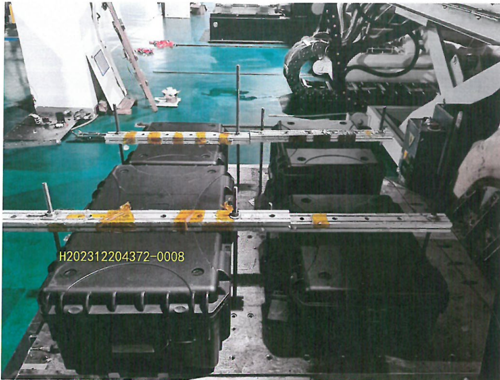
Attached figure 2.5 The vibration test is typically set up by the sample-Y axis (H202312204372-0008)
