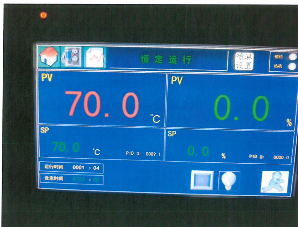
Attached figure 2.2 Temperature shock test equipment running interface - high temperature box (H202312204372-0007)
