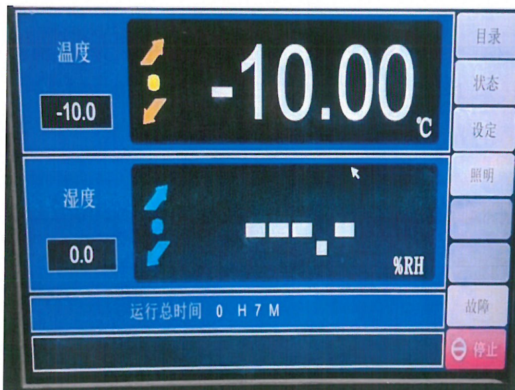
Attached figure 2.4 Temperature shock test equipment running interface-cryogenic box (H202312204372-0007)
