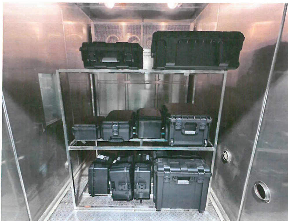
Attached figure 2.1 Temperature shock test subject placement diagram (H202312204372-0007)
