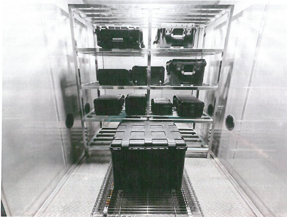
Attached figure 2.3 Temperature impact test subject placement diagram (H202312204372-0007)
