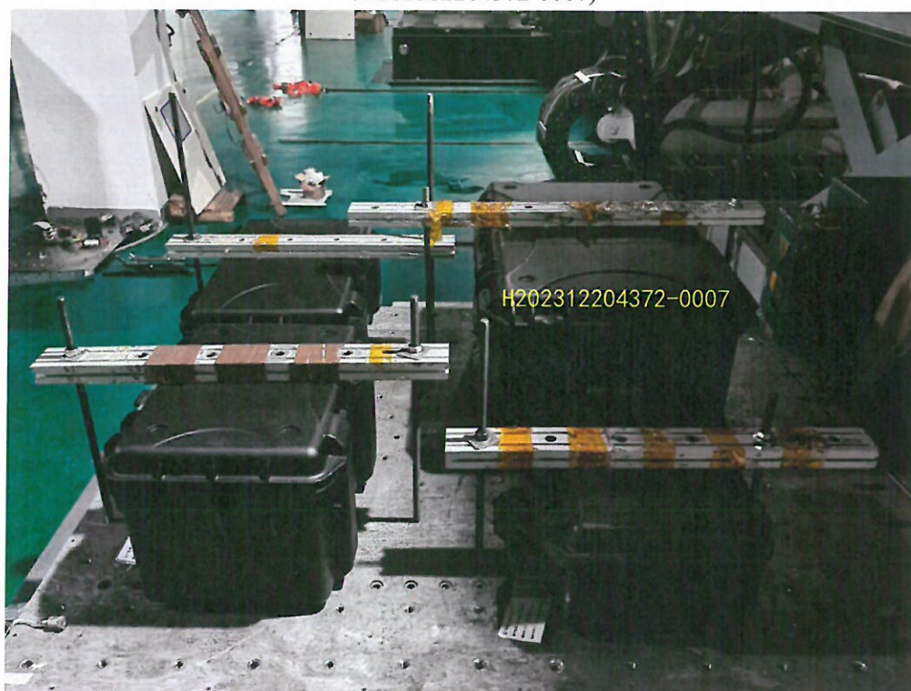
Attached figure 2.6 The vibration test is typically set up by the sample-Y axis (H202312204372-0007)
