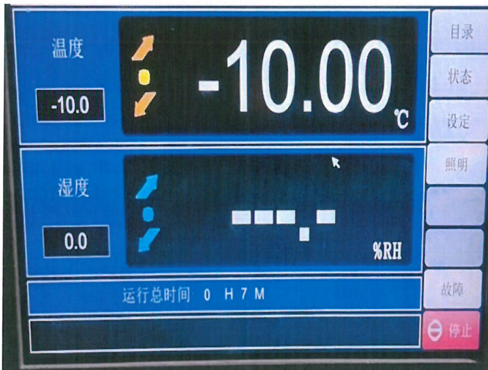
Attached figure 2.4 Temperature shock test equipment running interface-cryogenic box (H202312204372-0005)
