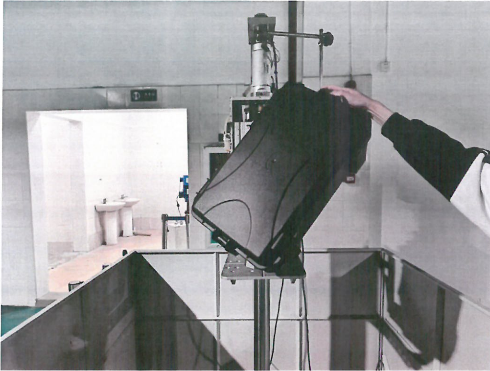
Attached figure 2.15 Drop test subjects set up typical graph-angles
