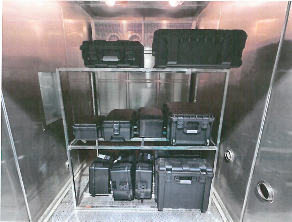
Attached figure 2.1 Temperature shock test subject placement diagram (H202312204372-0005)
