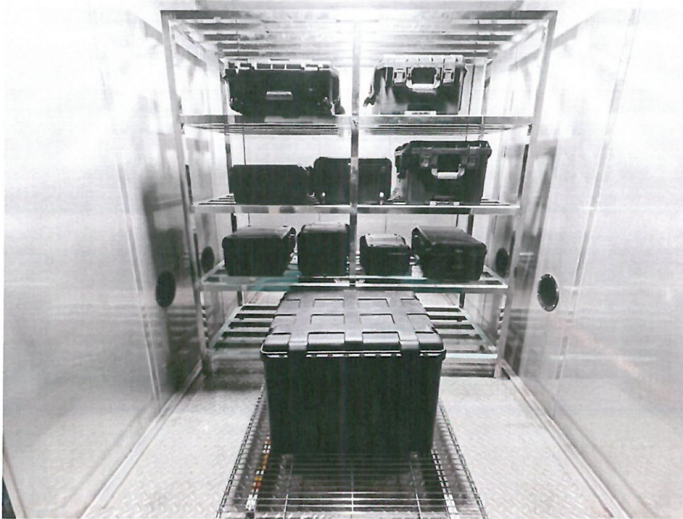
Attached figure 2.3 Temperature impact test subject placement diagram (H202312204372-0005)
