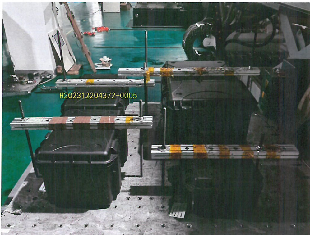
Attached figure 2.6 The vibration test is typically set up by the sample-Y axis (H202312204372-0005)
