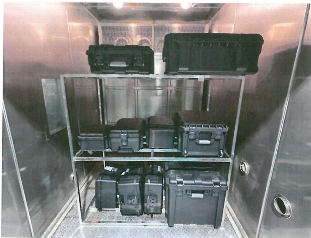
Attached figure 2.1 Temperature shock test subject placement diagram (H202312204372-0006)
