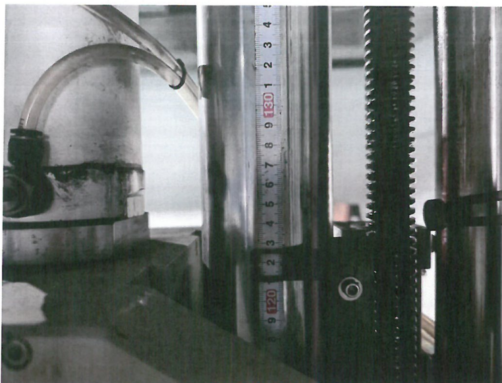
Attached figure 2.17 drawing of drop height 122cm (H202312204372-0006)
