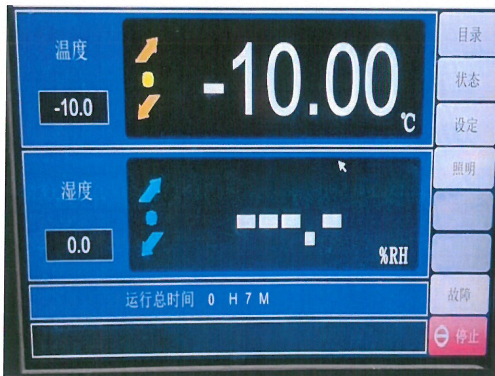
Attached figure 2.4 Temperature shock test equipment running interface-cryogenic box (H202312204372-0006)
