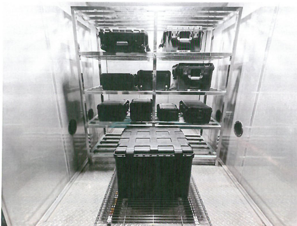
Attached figure 2.3 Temperature impact test subject placement diagram (H202312204372-0006)
