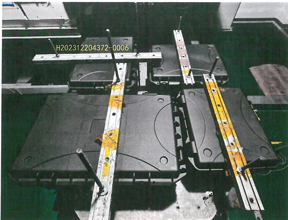
Attached figure 2.7 The vibration test is typically set up by the sample-Z axis (H202312204372-0006)
