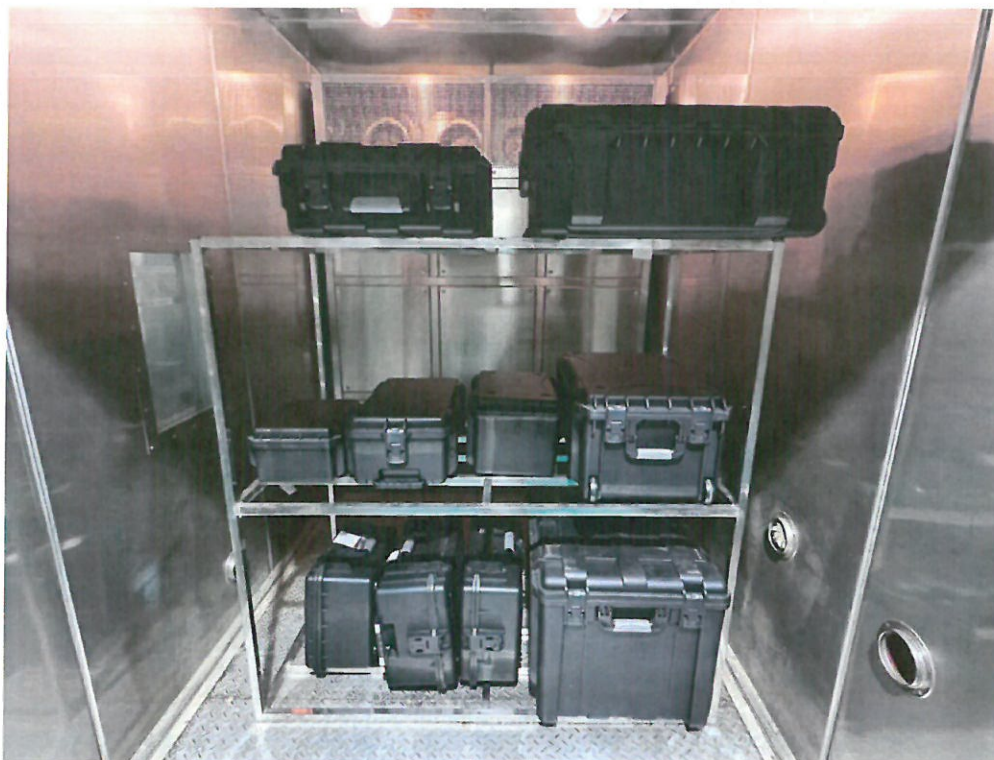
Attached figure 2.1 Temperature shock test subject placement diagram (H202312204372-0003)
