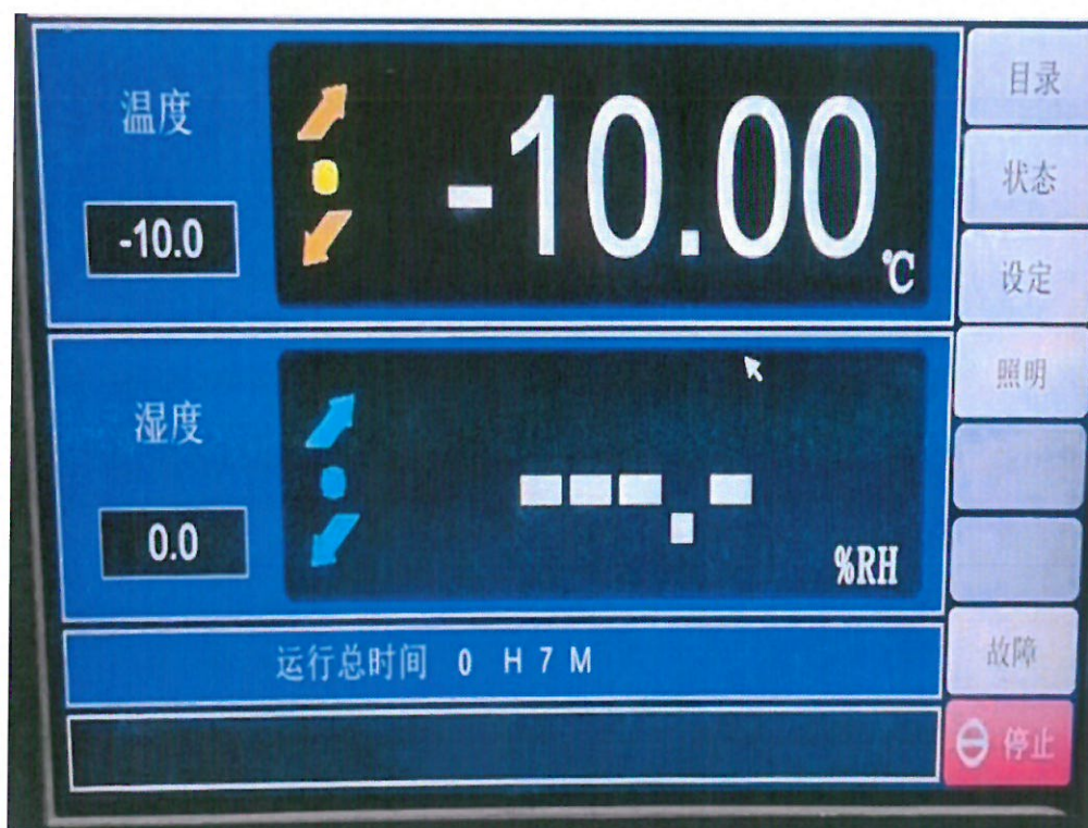
Attached figure 2.4 Temperature shock test equipment running interface-cryogenic box (H202312204372-0003)
