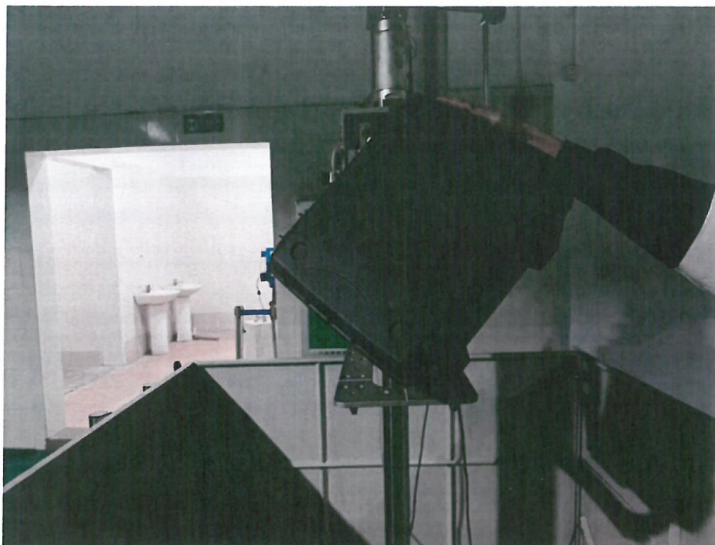
Attached figure 2.15 Drop test subjects set up typical graph-angles
