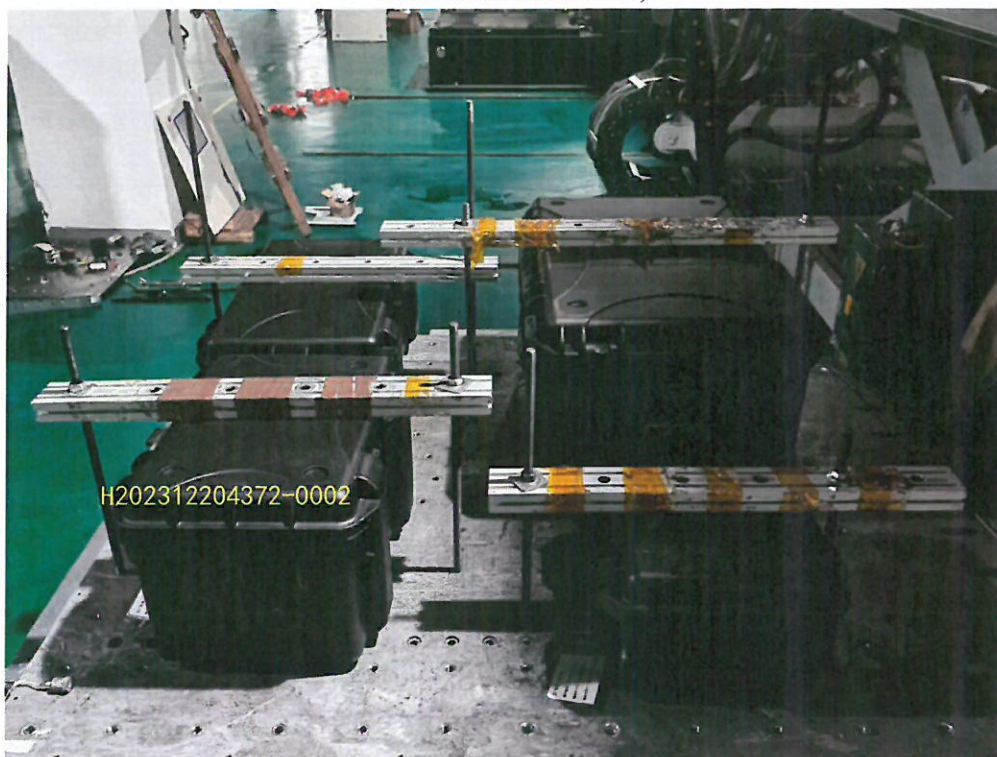
Attached figure 2.5 The vibration test is typically set up by the sample-Y axis (H202312204372-0002)
