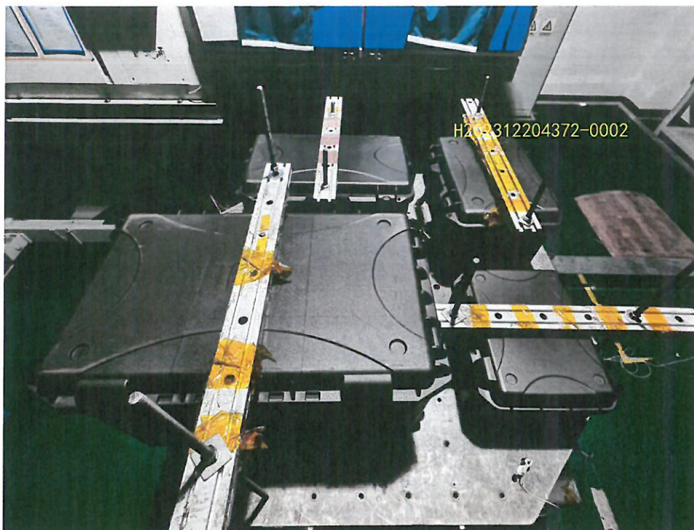
Attached figure 2.5 The vibration test is typically set up by the sample-Z axis (H202312204372-0002)
