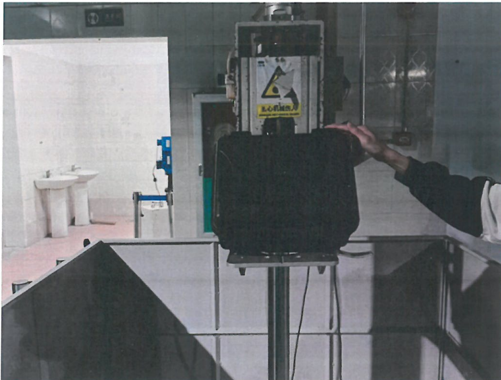
Attached figure 2.14 Drop test subjects erection typical diagram - Edge
