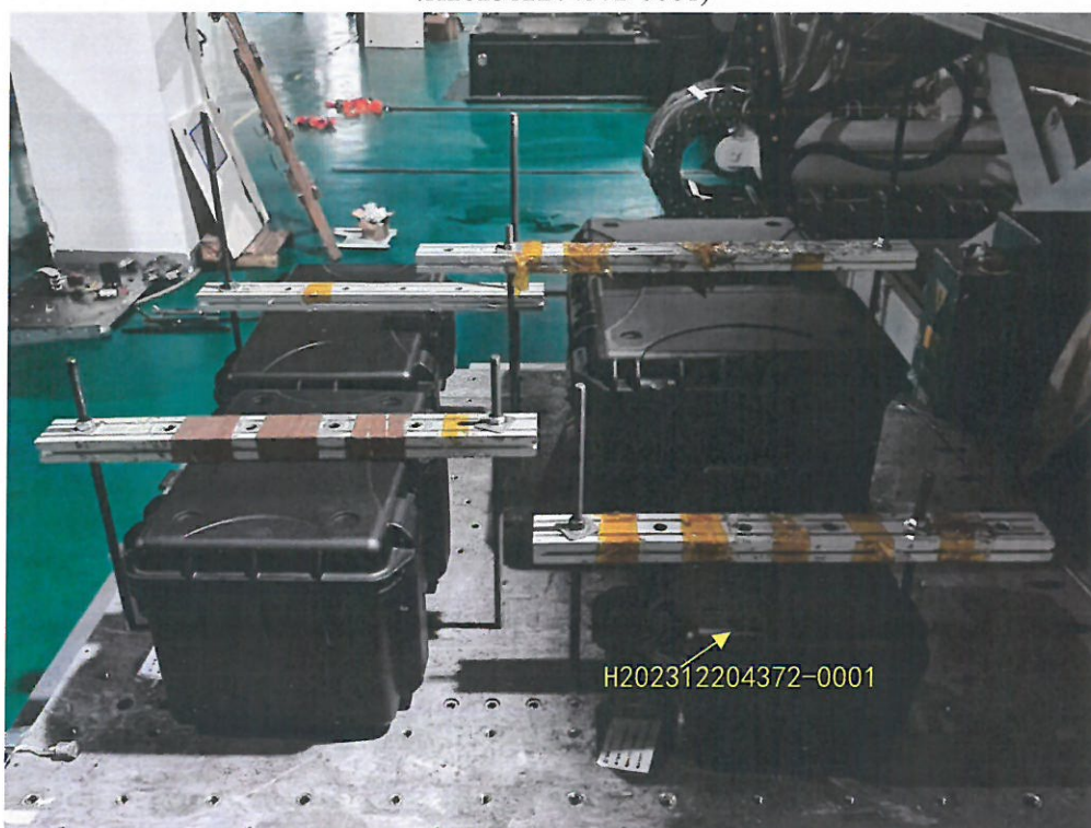
Attached figure 2.6 The vibration test is typically set up by the sample-Y axis (H202312204372-0001)
