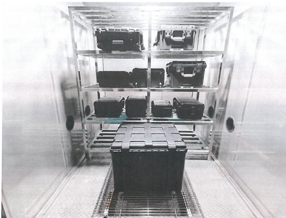
Attached figure 2.3 Temperature impact test subject placement diagram (H202312204372-0001)
