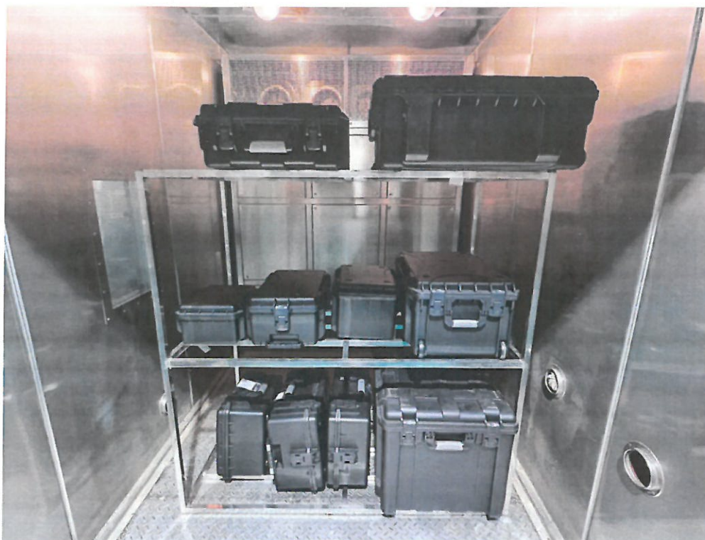
Attached figure 2.1 Temperature shock test subject placement diagram (H202312204372-0001)
